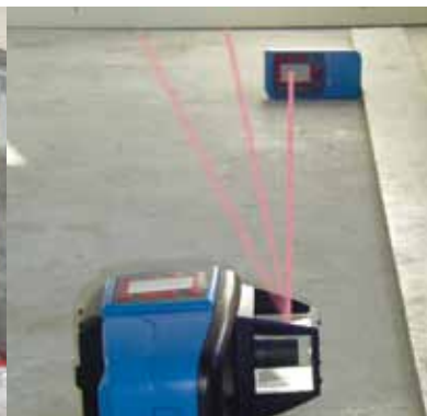
Align function using "search-and-align"
